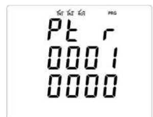
Potential Transformer Ratio
