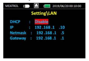
**Configuration LAN for MODBUS-TCP**
