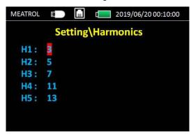
Could measure 5 different times harmonic value A or V. Setting times range: 2 to 51 times.
